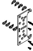
**Solution 2:** a plate with spacers + holder (suitable for foam fixing)
